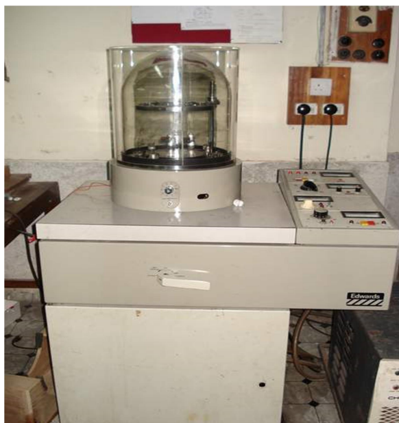
Fig. 3. The Edward vacuum coating unit E 306.
